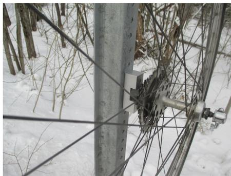
Step 3. While gripping the rim and tire, press down on the wheel to ensure that the dogs remain stationary as you turn the wheel counterclockwise.
